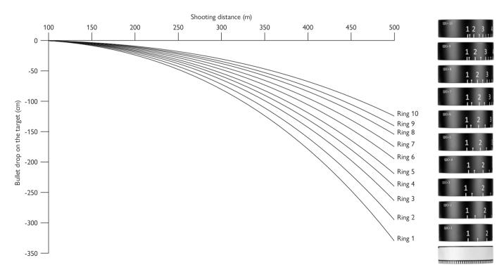
The ballistics calculator tells you the appropriate ring and provides a clear illustration of the trajectory.
